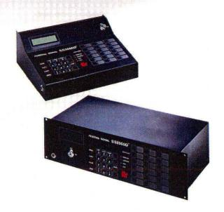
Federal Signal's SS2000 encoder is a versatile, user-friendly control unit. Available in one-way control and two-way status monitoring, the controller is offered in DTMF or AFSK formats. Encoded command sequences are field programmable and stored in memory for retention even when electrical power is removed. Federal Signal's SSLOADER offers an easy Windows®-based software package for configuring the encoder's command sequences and operating parameters.
